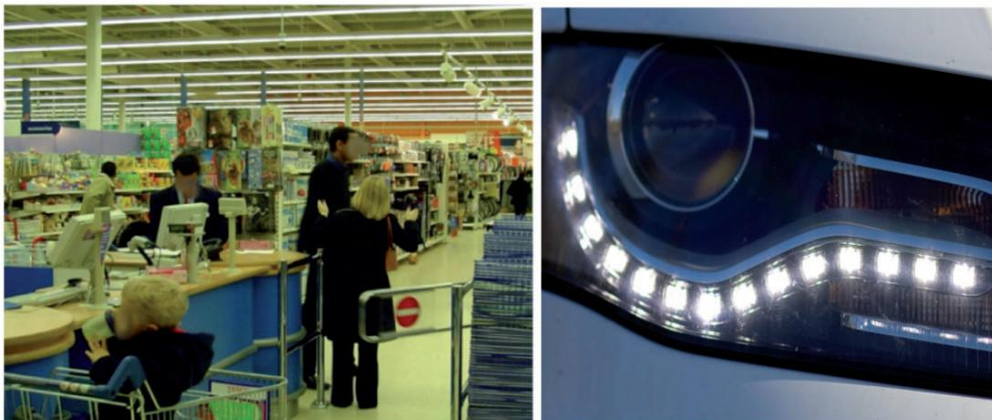
**Figure 5.** Uncomfortable configurations of luminaires and lamps (a) supermarket (b) daytime running light.
