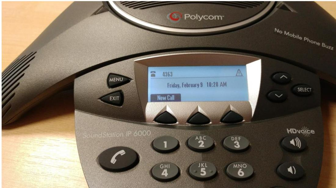
**2.29** To place a call please press the black triangular button under where the screen displays 'New Call' and dial as usual, either an internal extension number or dial 9 first for outside line then external number.
