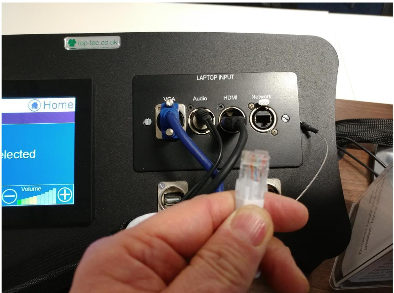
Please remove this network lead by first pinching the top and bottom between finger and thumb then gently pulling out.
